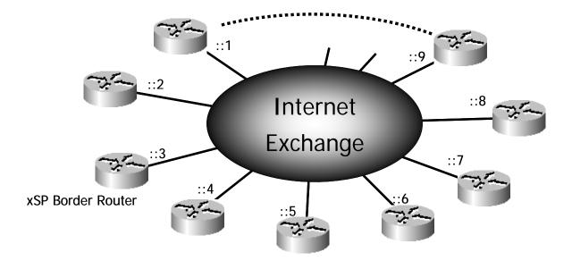
In the case of IX, a router for external connection is connected for each ISP on the same LAN segment. An address in the same subnet (A:B:C:D::/64 in Fig. mentioned above), which is allocated according to the policy of IX operator is assigned to connection interface of each router to IX.
