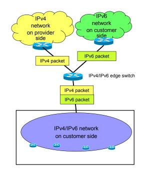
IPv6/IPv4 dual stack method (full replace type)
