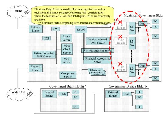
The local government building is to be changed over to Layer 2 as far as practicable in the interior. Then, the IPv6 multicast is to be distributed to PCs. IPv6 over IPv4 tunneling is implemented on the circuit between a branch and the local government building so that the IPv6 multicast distribution will be performed by way of the existing IPv4 infrastructure.
