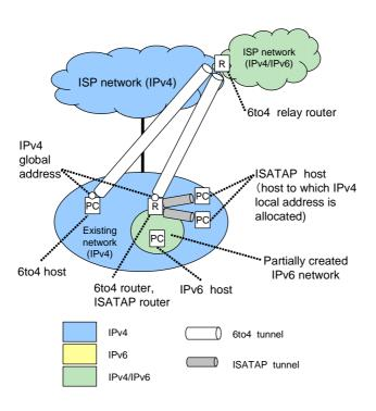
6to4 tunnel shall be created between disclosed 6to4 relay router and router/host that has IPv4 global address. Between ISATAP router (IPv4 global and local boundaries) and host that does not have IPv4 global address, ISATAP tunnel shall be created.
