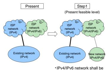
IPv4/IPv6 network shall be constructed independently from existing IPv4 network.
