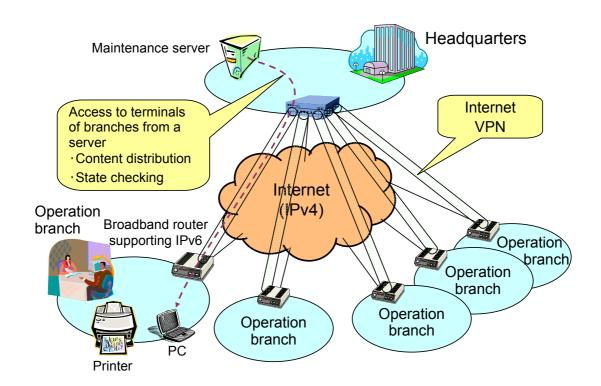
In this solution, IPv4 communication for business use and IPv6 communication for maintenance of operation branches are put through on Internet VPN. In the network of the headquarters, only the segment of the maintenance server is changed to support IPv6 and other segments inside the company are left as they are. IPv6 communication of maintenance server is performed from a gateway set in the headquarters using "IPv6 over IPv4 tunneling".
